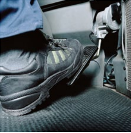
The accelerator is an electronic suspended pedal. It relieves the foot and provides a completely different driving sensation compared to floorbound mechanical pedals.
